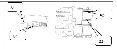
① The A1 and B1 sides of the RJ45 correspond to the A2 and B2 sides of the cable clip respectively.
